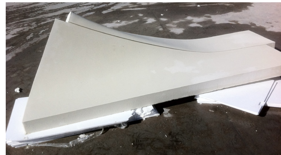
Mock Up – False Joint & Curvature
