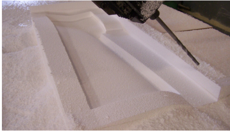
Fabrication – Milling Test Forms
