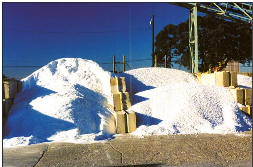
**Figure 6. For consistent, lasting color throughout the entire depth, white fine and coarse aggregates are the best choice. (70173)**
